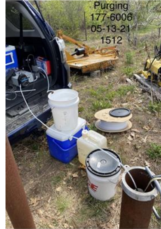
Monitoring well sampling
