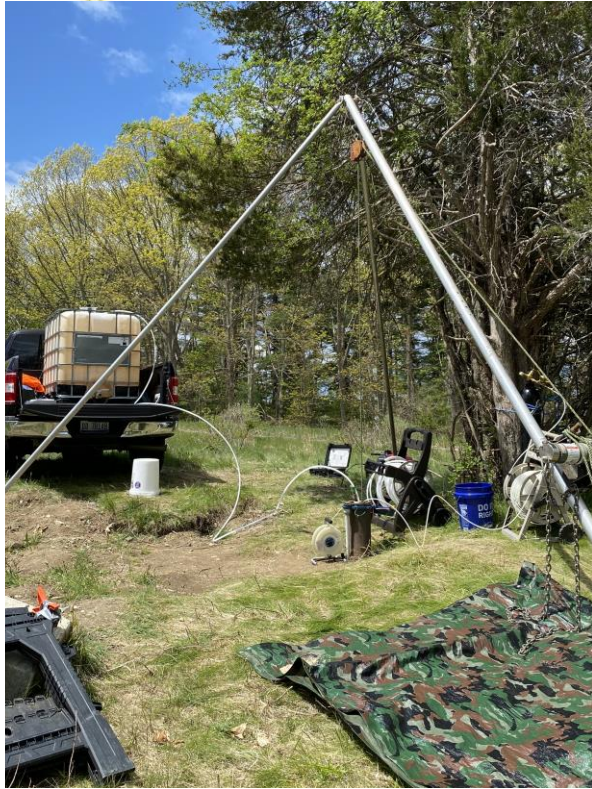
Deep bedrock well packer sampling
